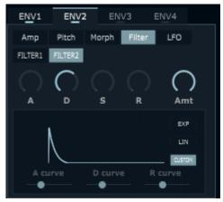
**FILTER1, 2**: Buttons to choose the filter cutoff modulated by the envelope.
